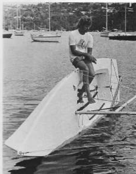
After a capsize, the Laser II comes up with a dry cockpit.
